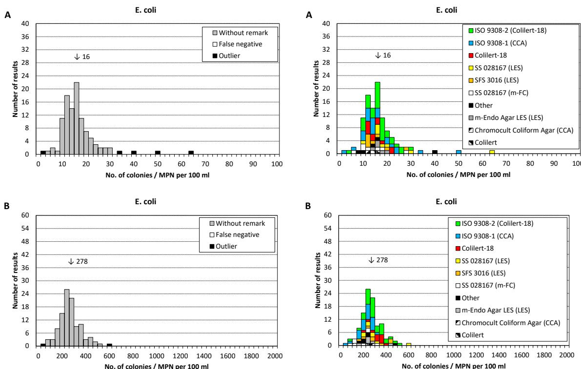
**Figure 3.** Results from analysis of *Escherichia coli*. The group "Other" includes the reporting of SFS 4088 (m-FC), m-FC Agar, ISO 9308-1:1990 (old edition, LES), NS 4792 (m-FC) and unknown methods.
