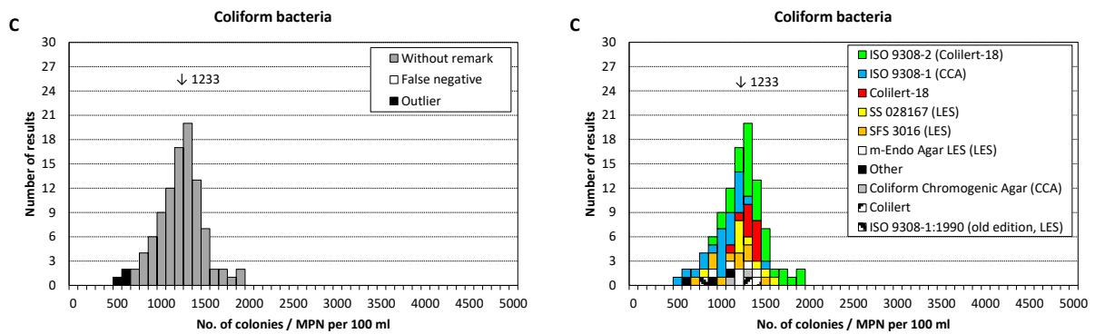
**Figure 1.** Results from analysis of coliform bacteria
