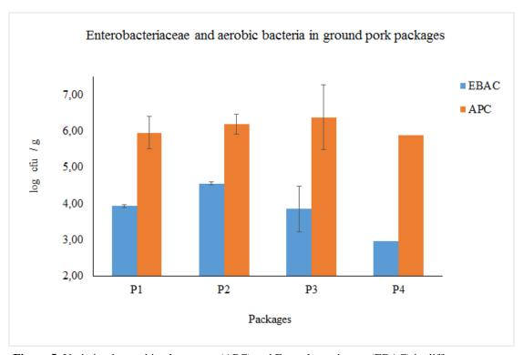
**Figure 5.** Variation in aerobic plate count (APC) and Enterobacteriaceae (EBAC) in different packages of ground pork. On the x-axis, package number is shown. One measurement was taken per ca 700 g meat, thus mean value of several measurements are shown for packages P1-P3, which weighed over 700 g. Standard deviation for each mean value is shown by error bars. *Results are variable, and especially interesting is the pronounced difference within package P3.*
