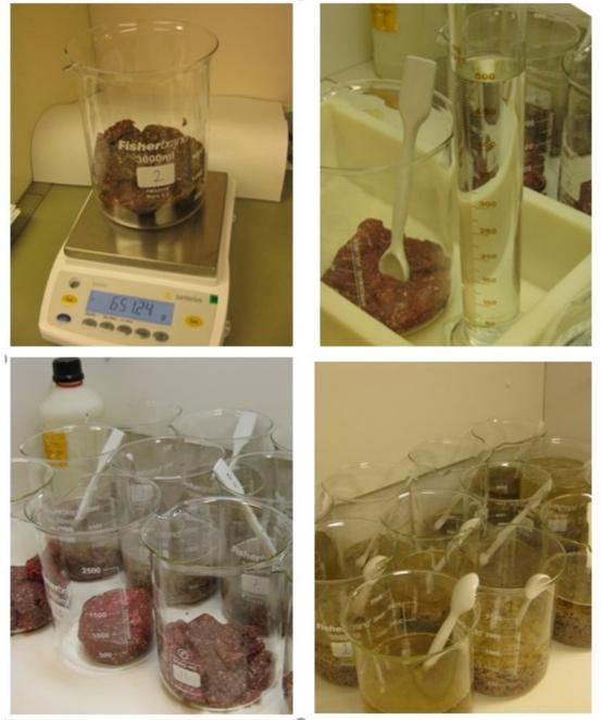
**Figure 2**. Sample preparation for extraction/dissolution of metal particles. Upper picture from the left: weighing in in 3 litre cups and the addition of 15 percent nitric acid. Lower picture from the left: minced moose meat before and after the addition of nitric acid.
