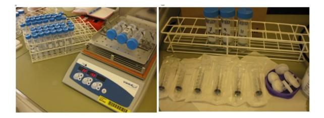
**Figure 4.** 8 mg of lead shavings were placed in 50 ml test tubes along with 40 ml of 0.1 M hydrochloric acid. Three samples, one of which was blank, were placed in a shaker machine and three in a test tube rack.
