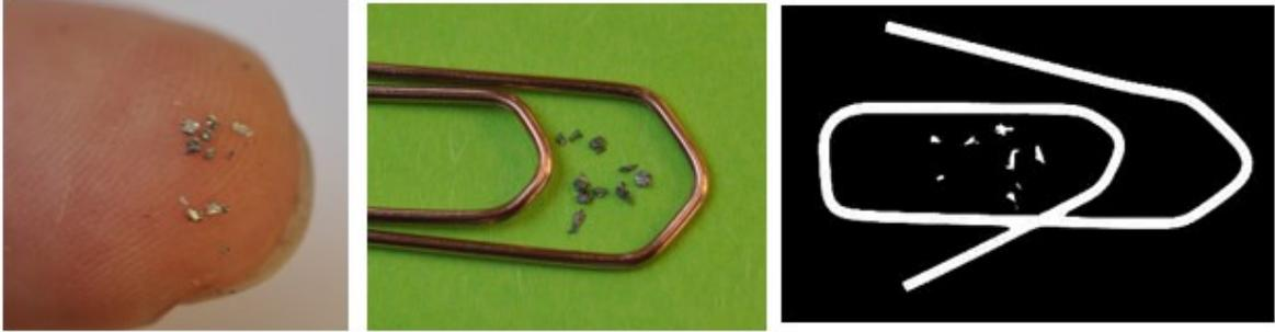
Figure 3. The pictures show 8 mg of lead shavings from a used lead bullet, photographed on a finger tip and alongside a paper clip. The black and white picture shows an x-ray image of a paper clip and 8 mg of lead shavings. The maximum permitted level for lead in meat from cattle, sheep, pigs and poultry is 0.1 mg/kg, which means that 8 mg contaminates 80 kg of meat up to the maximum permitted level. Photograph: SVA, 2014.
