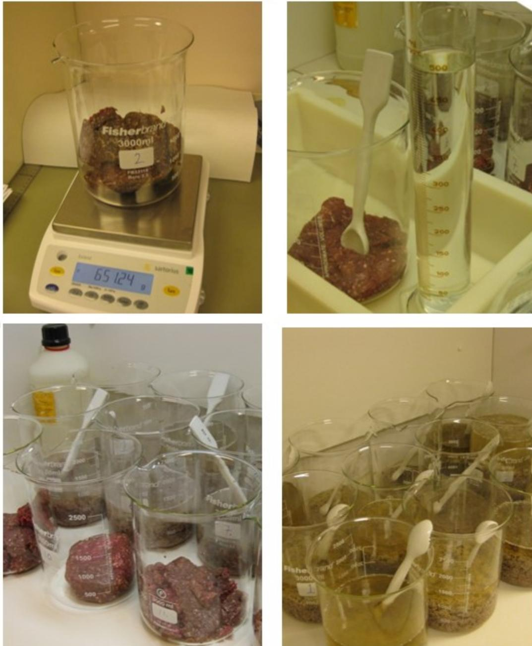
**Figure 2.** Sample preparation for extraction/dissolution of metal particles.
