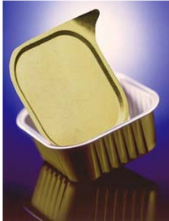
Figure B7.4.d. Typical PET-food container lacquered outside; laminated with CPP inside with thermo-sealable lid (inside CPP coextruded and outside lacquered and, possibly, printed)
