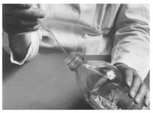
**9.** Transfer the suspension to the bottle containing 100 ml diluent.
