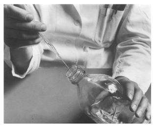
6. Repeat steps 4 and 5 three more times with the same pasteur pipette. Rinse the walls of the vial carefully. After thorough intermittent mixing, for a minimum of 3 minutes (even better >10 min), the sample is ready for analysis. Perform the analyses within 60 min.
