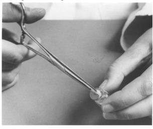
**3**. Remove the rubber plug. Carefully burn off the opening of the vial over a gas flame.
