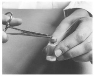
1. Twist the flap on the upper side of the aluminium cap in the direction of the arrow. Use a pair of forceps, tweezers or similar.
