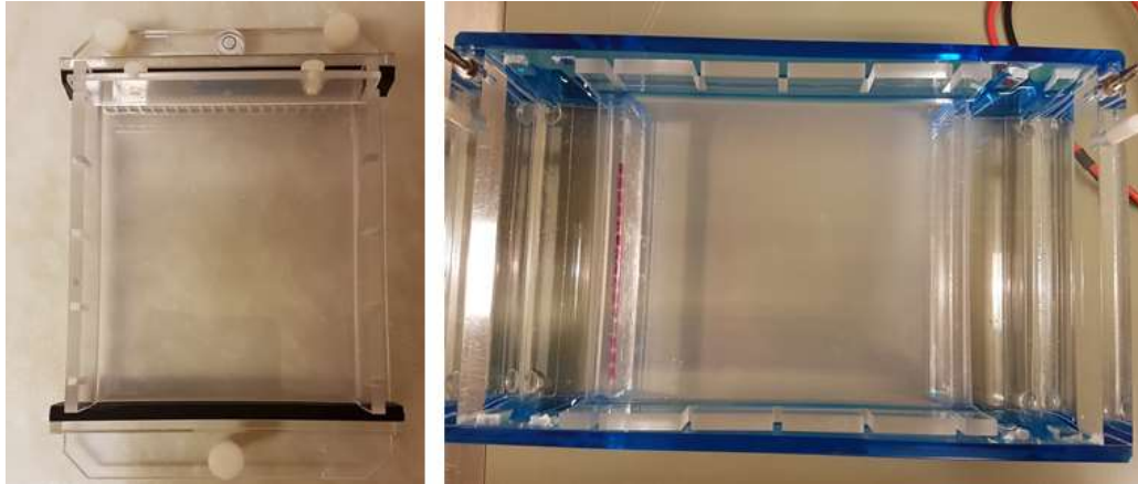
Fig. 1. Preparation of an agarose gel. Left: gel rig, right: a loaded agarose gel in an electrophoresis tank filled with TBE buffer
